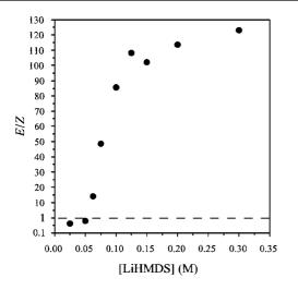
*Figure 1.* E/Z selectivity (*E*-6:*Z*-6, eq 3) versus molarity (M) of LiHMDS in samples containing 0.10 M ketone 5 and 1.2 M excess Et<sub>3</sub>N in toluene at -78 °C.<sup>16</sup>
