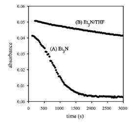
Figure 4. IR absorbance of enolate 15 versus time in (A) 1.5 M  $Et_3N/t$  toluene and (B) 1.5 M  $Et_3N/1.5$  M THF/toluene.
