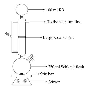
The Schlenk flask was cooled to 0 °C, and BuLi was added via syringe followed by dropwise addition of HMDS. After stirring 30 min, the solution was warmed to rt and stirred an additional 30 min.
